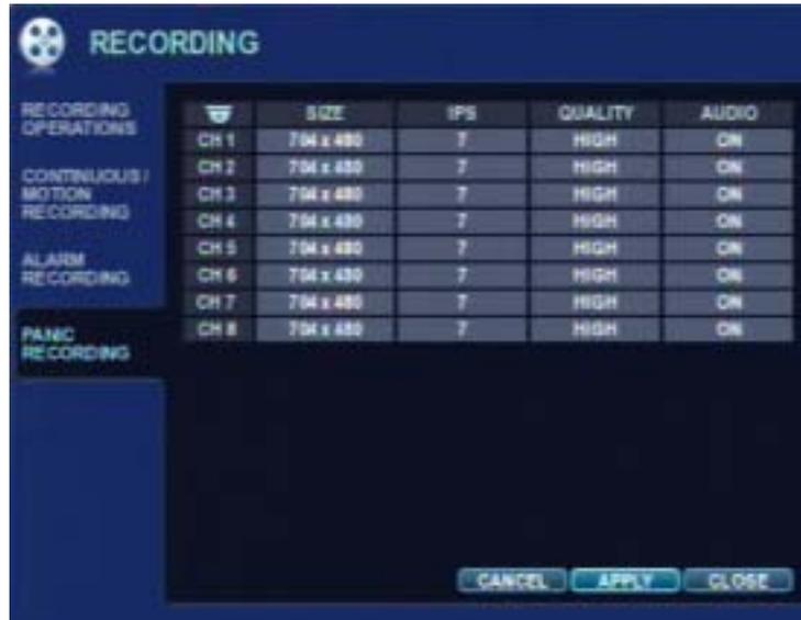
During Panic Recording, the DVR overrides all other recording settings and uses the settings configured here to record continuously on all channels.
