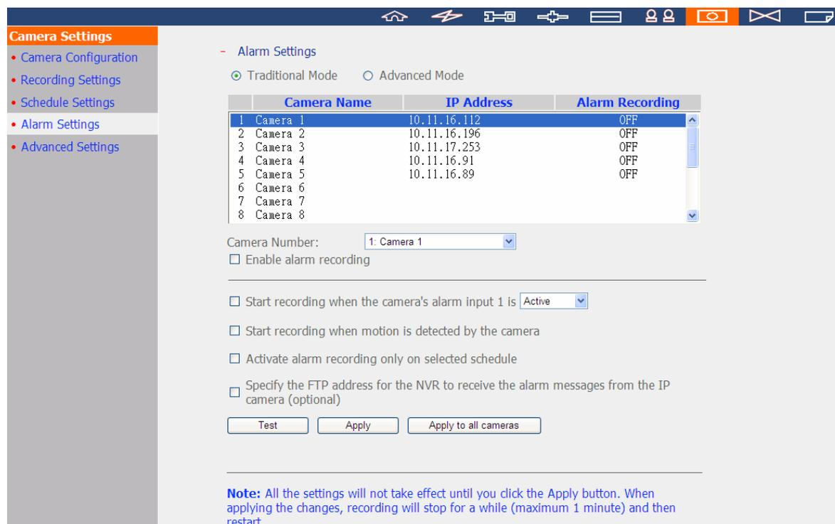
The screenshot displays the "Camera Settings" interface for "Alarm Settings" in "Traditional Mode". A table lists 8 cameras with their names and IP addresses, and their alarm recording status is currently "OFF". Below the table, there are several configuration options for the selected camera (Camera 1):
