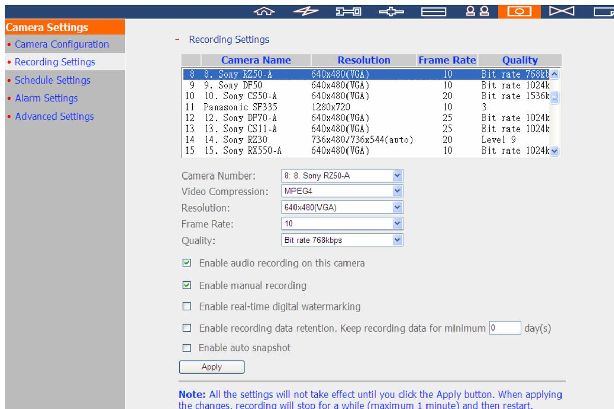
The screenshot displays the 'Camera Settings' window, specifically the 'Recording Settings' tab. On the left, a sidebar lists navigation options: Camera Configuration, Recording Settings (selected), Schedule Settings, Alarm Settings, and Advanced Settings. The main area shows a table of cameras and their recording parameters, followed by configuration fields and checkboxes.
