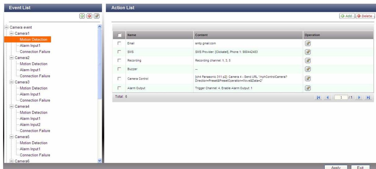
The screenshot displays two windows from the NVR interface. The 'Event List' window on the left shows a tree view of events for six cameras. Under 'Camera1', 'Motion Detection' is selected. The 'Action List' window on the right shows a table of actions defined for the selected event.
