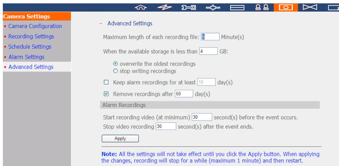
The screenshot displays the 'Advanced Settings' interface for a camera. On the left, a sidebar lists navigation options: Camera Configuration, Recording Settings, Schedule Settings, Alarm Settings, and Advanced Settings (which is currently selected). The main content area is titled 'Advanced Settings' and includes the following configuration options:
