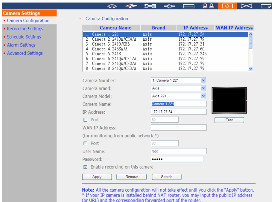
The screenshot displays the 'Camera Configuration' interface. On the left, a sidebar lists settings: Camera Configuration (selected), Recording Settings, Schedule Settings, Alarm Settings, and Advanced Settings. The main area shows a table of camera configurations:
