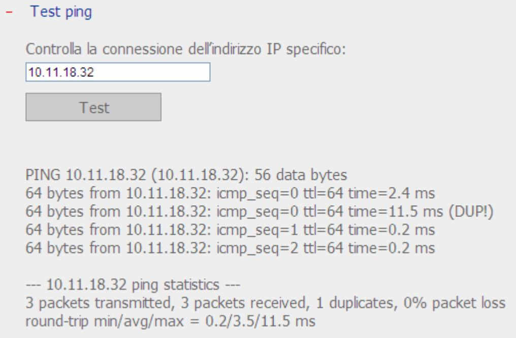
The screenshot shows a window titled "Test ping" with a subtitle "Controlla la connessione dell'indirizzo IP specifico:". Below the subtitle is a text input field containing "10.11.18.32" and a "Test" button. The output of the ping test is displayed below the button:
