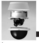
**1.** Remove the camera's outer cover and ceiling panel.
