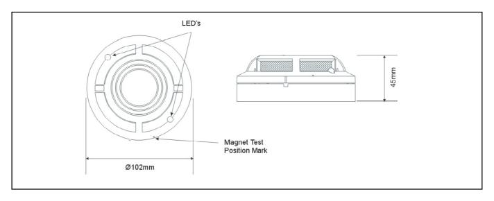
Each sensor base includes a tamper resistant option which, when activated, prevents the removal of the sensor from its base without the use of a tool. Full circuit functionality can be easily confirmed on site by use of the sensor test switch. Operation of this magnetic switch will generate an alarm response to the fire alarm control panel, making system testing both convenient and simple.
