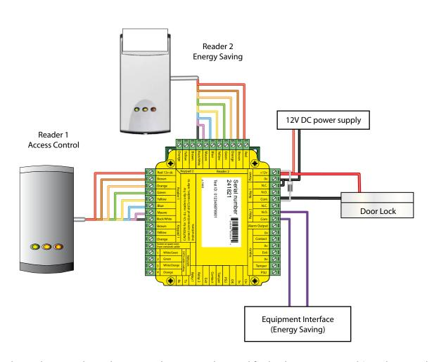
The above diagram shows how a single ACU can be used for both access control (Reader 1 - Relay 1) and energy saving (Reader 2 - Relay 2).
