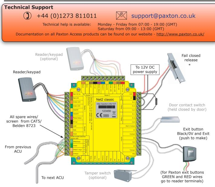
\* For a fail open lock (Maglock), the 0V link wire must be connected to the "NC" terminal.
