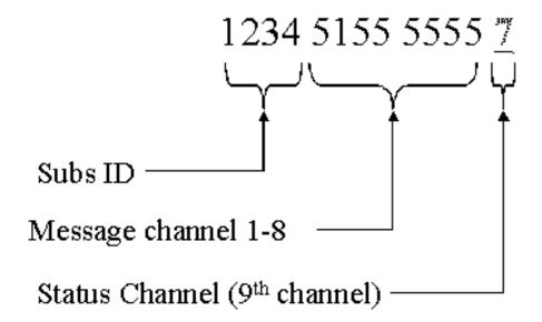
"Single Round with Checksum" sends one message, using a checksum digit for verification:
