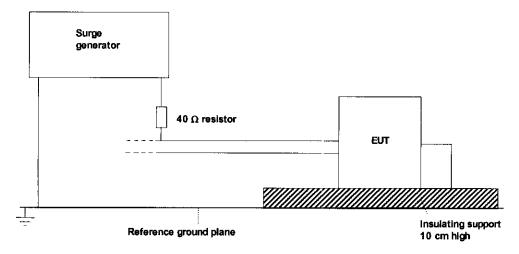
Application on D.C. mains and signal lines (unshielded cables)
