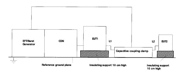
L1 : 1 m L2 : 1 m when both EUT are tested 5 m when only EUT1 is tested
